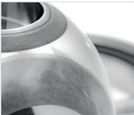
Ball surface plating with 150 micron TCC.
